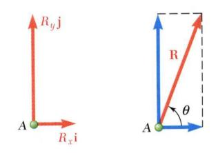
• The scalar components of the resultant are equal to the sum of the corresponding scalar components of the given forces.
