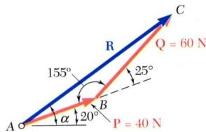
• Trigonometric solution - Apply the triangle rule. From the Law of Cosines,
