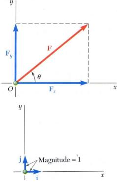
• May resolve a force vector into perpendicular components so that the resulting parallelogram is a rectangle.  $\vec{F}_x$  and  $\vec{F}_y$  are referred to as *rectangular vector components* and
