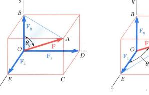
• With the angles between  $\vec{F}$  and the axes,
