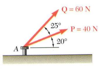
Graphical solution - A parallelogram with sides equal to P and Q is drawn to scale. The magnitude and direction of the resultant or of the diagonal to the parallelogram are measured,
