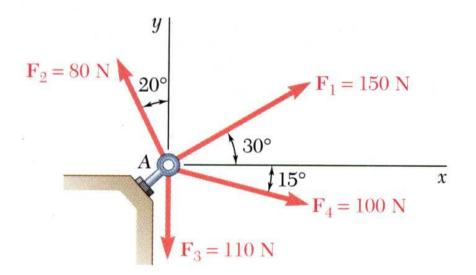
Four forces act on bolt *A* as shown. Determine the resultant of the force on the bolt.
